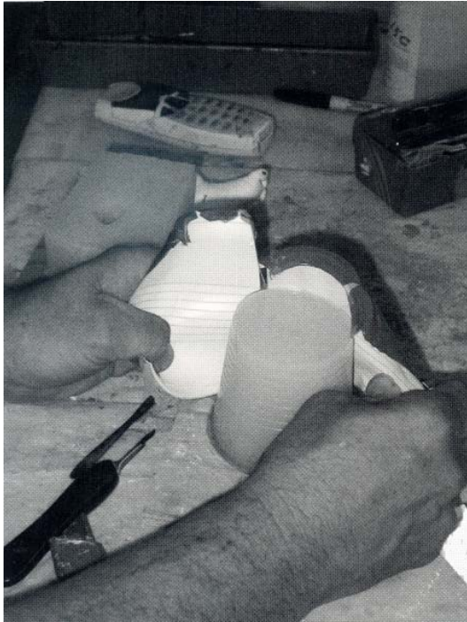
Removing the cup from the hand mold Notice the enlarged hole on top of the foot mold.
