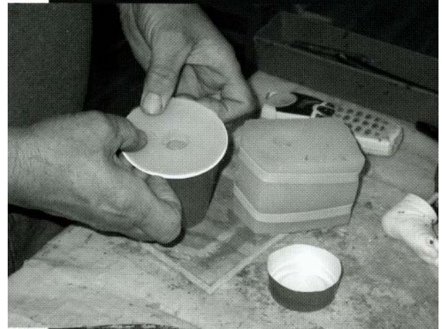
Fitting the hand mold into a new cup which has had its bottom removed. Notice rubber bands around the foot mold.
