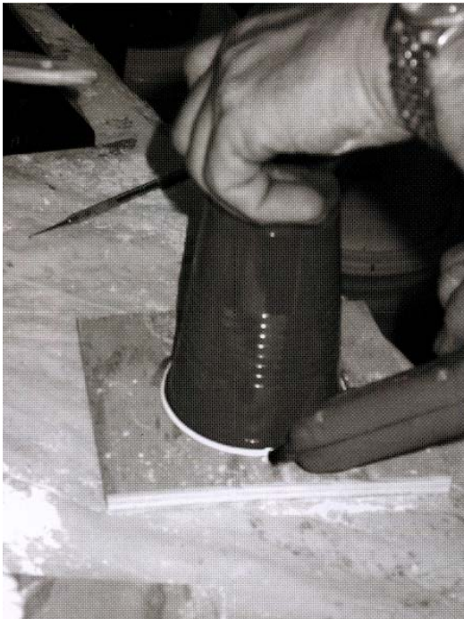
Attaching the cup to the base with a hot glue gun:
