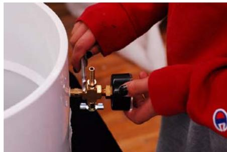
Photograph #4: Attaching the copper valve to the pre-threaded hole in the vacuum chamber
