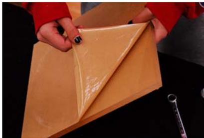
Photograph #7: Peeling off the protective paper from the acrylic sheets
