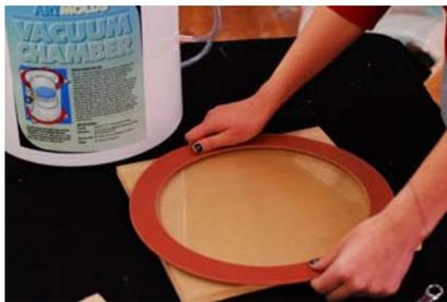
Photograph #8: Positioning the bottom gasket
