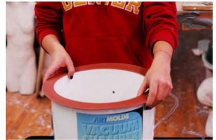
Photograph #10: Placing the top gasket in place
