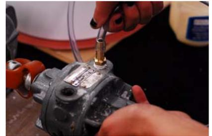
Photograph #12: Connecting the plastic tube directly to the vacuum pump
