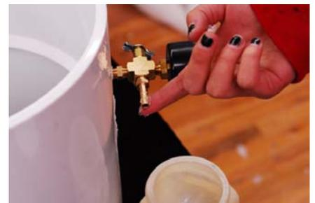
Step 1: In photo #3, Stevie was attaching the vacuum gauge to the brass fitting.
