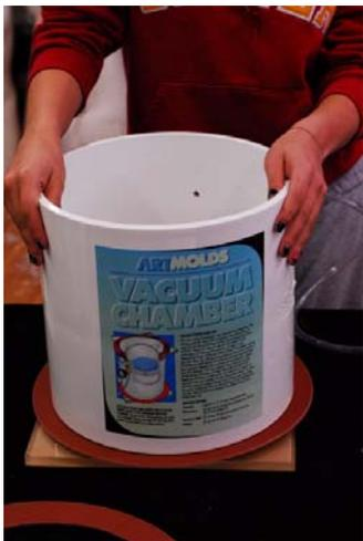
Photograph #9: Setting the vacuum chamber on the bottom gasket
