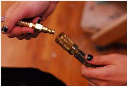
Photograph #14: The plastic tub can be attached to the vacuum line with a quick disconnect coupling
