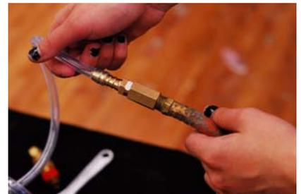
Photograph #13: Plastic tube connected to the vacuum hose with a barbed fitting
