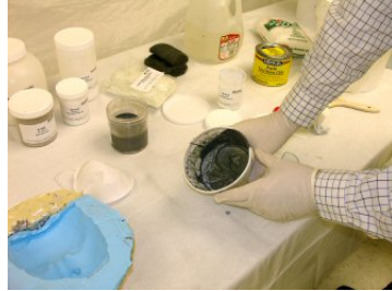
Step 8 You will notice the face mix begins to thicken when you mix in the accelerator.
