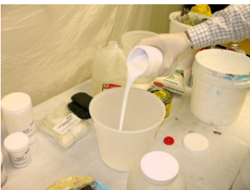
Step 15 Begin mixing the backup mix by pouring the backup VF-812 into a clean mixing container.
