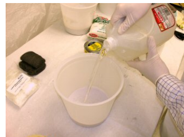
Step 18 Add about 6 tablespoon of accelerator. But be careful not to add too much or your backup mix will set before you have a chance to apply it.
