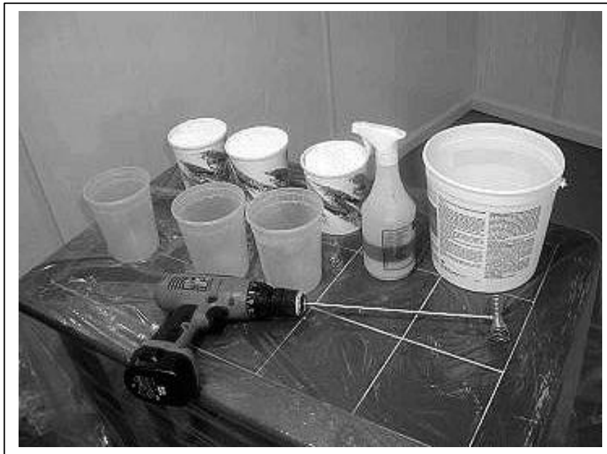
A lifecaster's setup preparing alginate for mold making. The three containers in the rear hold alginate powder. The large bucket on the right holds the water. The empty containers in the front will be used to combine the alginate and water.
